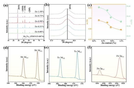
Fig. 2 (a) XRD patterns of the synthesized Zn-doped thin film samples with pristine  $Sb_2Te_3$  from 10° to 80°; (b) the enlarged XRD patterns of the (015) diffraction peak; (c) the development of lattice parameters a and c with increasing Zn content; XPS spectra of Zn-doped  $Sb_2Te_3$  samples and Gaussian-fitted valence states in XPS spectra: (d) Sb 3d, (e) Te 3d, and (f) Zn 2p.
