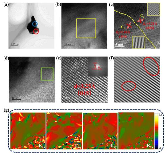
Fig. 4 (a) Low-resolution TEM image of the Zn 0.58% Sb<sub>2</sub>Te<sub>3</sub> sample; (b) HR-HAADF image of the blue circled area in (a); (c) HR-TEM image of the rectangular area in (b) with the inset of the IFFT images; (d) HR-TEM image of the red circled area in (a); (e) atomic scale HR-TEM image of the rectangular area in (d) with the inset of the FFT image; (f) IFFT image of (e) with lattice distortion; (g) strain/distortion maps by GPA analysis in (e).
