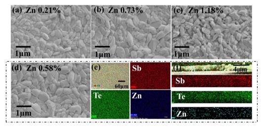
Fig. 3 SEM images of the surface morphology in (a) Zn 0.21%, (b) Zn 0.73%, (c) Zn 1.18%, and (d) Zn 0.58%  $Sb_2Te_3$  thin film samples; (e) EDS mapping image of the Zn 0.58% sample surface with Sb, Te, and Zn and the distribution of all three elements; (f) EDS mapping image of Zn 0.58% sample cross-sectional area with Sb, Te, and Zn and the distribution of all three elements.
