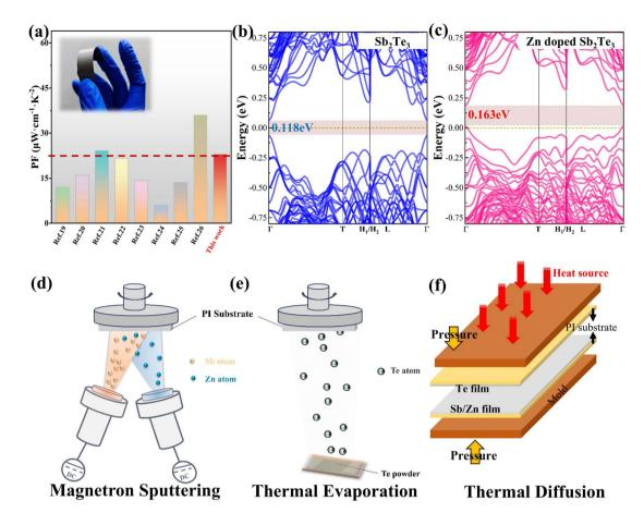
Fig. 1 (a) Comparison of PF values with those in the references; calculated band structures of the (b) pristine and (c) Zn-doped Sb<sub>2</sub>Te<sub>3</sub> material by DFT calculations; (d) schematic diagram of the fabrication process of a Sb/Zn precursor thin film by magnetron sputtering; (e) schematic diagram of the fabrication process of a Te precursor thin film by thermal evaporation; (f) schematic diagram of the thermal diffusion process using Sb/Zn and Te precursor thin films.
