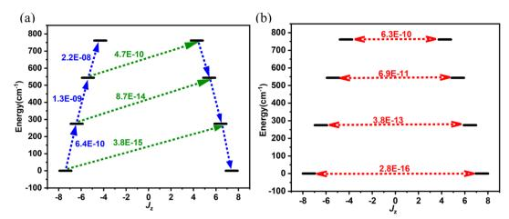
Fig. 3 (a) Orbach transition rates computed at 20 K and (b) Raman transition rates computed at 6 K. The Orbach transition rates show the matrix elements of,  $\hat{W}^{1-ph}$  whereas the Raman relaxations show the matrix elements of  $\hat{W}^{2-ph}$ . Rates are expressed in ps<sup>-1</sup> and only rates larger than  $10^{-16}$  are reported explicitly. The x-axis displays the computed average magnetic moment for the first four KDs and their energy separation from the ground state.
