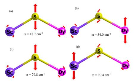
Fig. 5 (a) First vibration of vib1, (b) second vibration of vib1 (c) first vibration of vib2 (d) second vibration of vib2. The red arrows indicate the movement, with the size of the arrow representing the extent of motion for that particular atom.
