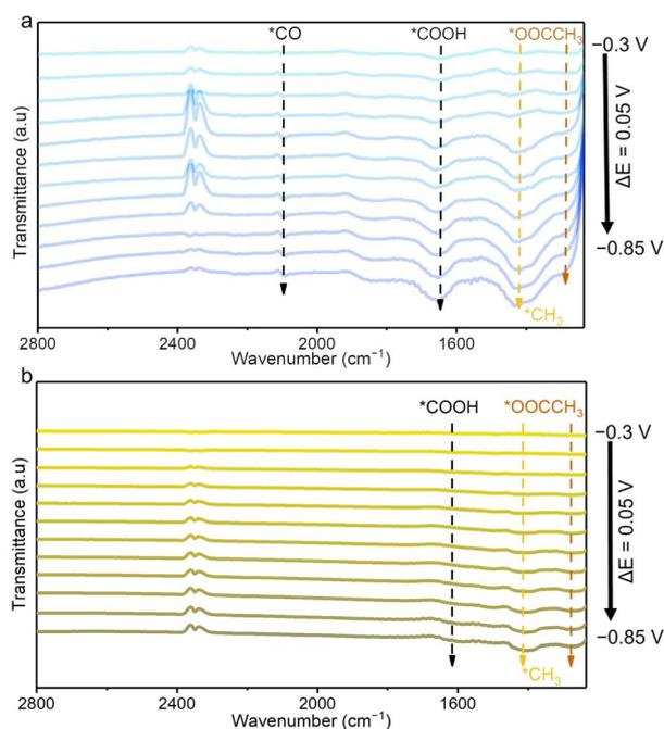
Fig. 4 *In situ* ATR-FTIR spectra of (a) Cu-Ag/NC and (b) Cu/NC under CO<sub>2</sub>RR conditions.
