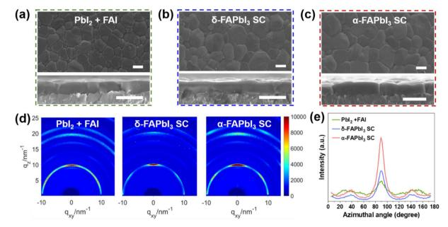
Fig. 2 Crystallinity of films based on different FAPbl<sub>3</sub> precursors. (a-c) Top-view (top) and cross-sectional (bottom) SEM images. Scale bars: 1 μm. (d) GIWAXS patterns and (e) derived azimuthal intensity profiles of the (100) peak of the FAPbl<sub>3</sub> perovskite films based on Pbl<sub>2</sub> + FAI, δ-FAPbl<sub>3</sub> and α-FAPbl<sub>3</sub> SCs.
