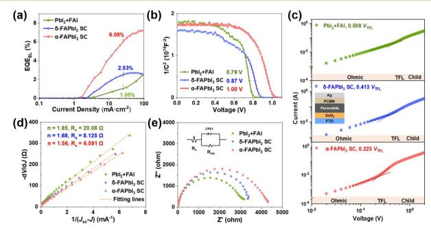
Fig. 4 Characterization of devices based on different FAPbl<sub>3</sub> precursors. (a) EQE<sub>EL</sub>-current density curves, (b) Mott–Schottky plots, (c) dark I-V characteristics from SCLC measurements of the electron-only devices (structure shown as inset), (d) relationship between -dV/dJ and  $(J_{sc}-J)^{-1}$  in dark and (e) EIS data (fitting circuit model as inset) of the devices based on Pbl<sub>2</sub> + FAI,  $\delta$ -FAPbl<sub>3</sub> and  $\alpha$ -FAPbl<sub>3</sub> SCs.
