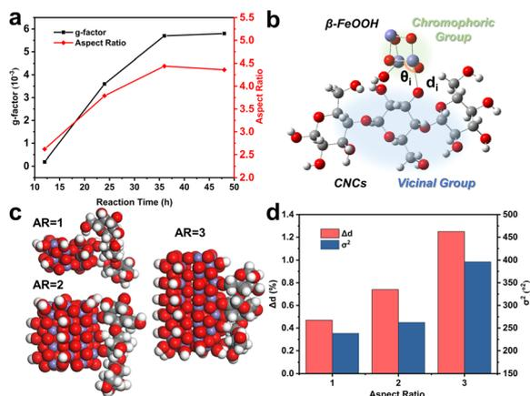
Fig. 4 (a) The change of the  $g$ -factor and ARs during the reaction. (b) Schematic illustration of the division of two groups in one-electron theory. (c) Space-filling models of iron oxide clusters with different ARs connected with  $\beta$ -1,4-linked anhydro-D-glucose from three monomers through Fe–O–C<sub>3</sub>. (d) The effect of ARs on  $\Delta d$  and  $\sigma^2$ .
