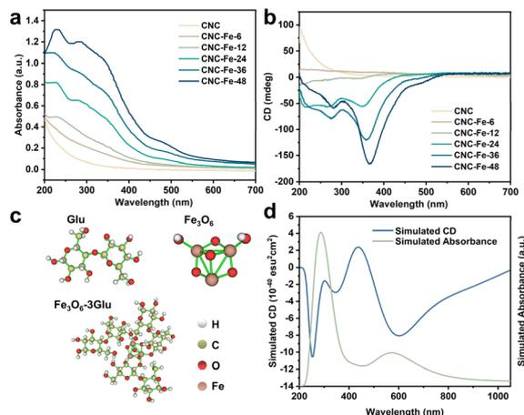
Fig. 3 (a) UV-vis and (b) CD spectra of dispersions of CNCs and CNC-Fe- $x$  ( $x = 6-48$ ). (c) Atomistic models used for TD-DFT calculations. (d) Simulated CD and absorption spectra of Fe<sub>3</sub>O<sub>6</sub>-3Glu.
