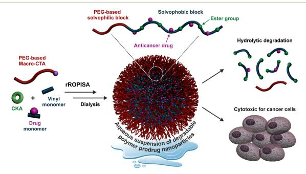
Fig. 1 Synthesis of aqueous suspensions of core-degradable diblock copolymer prodrug nanoparticles by radical ring-opening polymerization-induced self-assembly (rROPISA) from cyclic ketene acetals (CKAs) and drug-bearing monomers.
