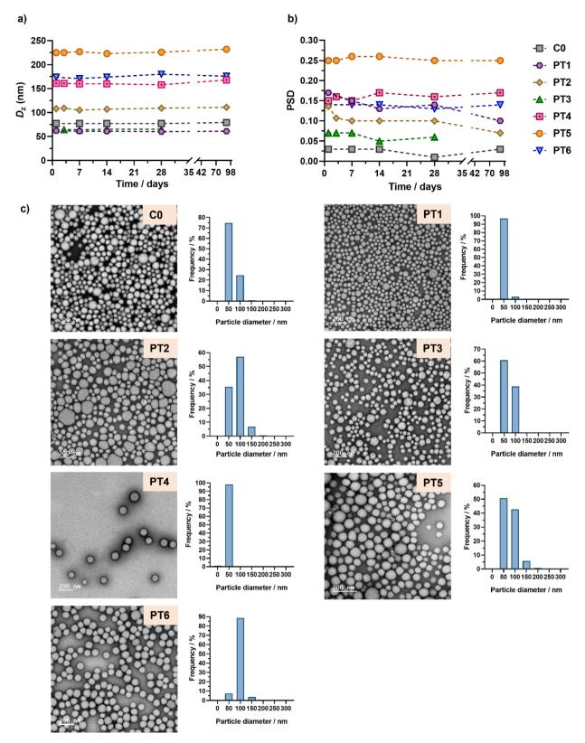
Fig. 3 Evolution with time of (a) the intensity-weighted mean diameters ( $D_z$ ) and (b) the particle size distributions (PSD) of POEGMA<sub>28</sub>-b-P(LMA-co-CKA-co-PtxMA) nanoparticles CO and PT1-PT6 determined by DLS after dialysis against water. (c) Representative TEM images and particle size distributions (n = 350-1000) of nanoparticles CO and PT1-PT6 determined by TEM ( $d_n$ ,  $d_w$ ,  $d_z$ , and polydispersity values are given in Table S3†).
