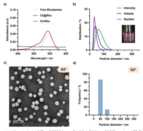
Fig. 7 (a) Absorption spectra of free rhodamine B (Rho), P(OEGMA<sub>24</sub>-co-RhoMA)-b-P(LMA-co-BMDO) copolymer (C0-Rho) and POEGMA<sub>28</sub>-b-P(LMA-co-BMDO) copolymer (C0@Rho). (b) DLS measurements of nanoparticles G2\*, giving average diameters expressed in intensity, volume and number. Inset: picture of the aqueous suspension of nanoparticle G2\*. (c) Representative TEM image and (d) particle size distributions (n = 750) of nanoparticles G2\*.
