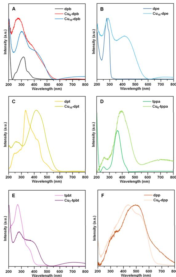
Fig. 6 Solid-state UV-vis absorption spectra of (A) dpb,  $\text{Cu}_6\text{-dpp}$ ,  $\text{Cu}_{10}\text{-dpp}$ , (B) dpe,  $\text{Cu}_{10}\text{-dpe}$ , (C) dpt,  $\text{Cu}_{10}\text{-dpt}$ , (D) tppa,  $\text{Cu}_6\text{-tppa}$ , (E) tpbt,  $\text{Cu}_7\text{-tpbt}$ , and (F) dpp,  $\text{Cu}_6\text{-dpp}$  at room temperature.
