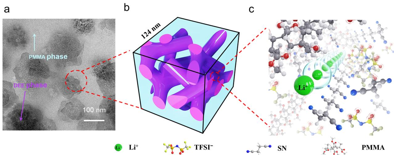
Fig. 6 Schematically illustrating the interconnected structure of elastomeric electrolytes prepared by denture-inspired *in situ* polymerization of MMA, with pipelines consisting of SN and LiTFSI that provide fast pathways for  $\text{Li}^+$  transfer. (a) Transmission electron microscopy images of  $\text{PM}_2\text{S}_3$ . (b) Interconnected pipeline structure of  $\text{PM}_2\text{S}_3$ . (c) Fast pathways for  $\text{Li}^+$  transfer.
