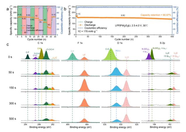
Fig. 3 Illustration of the performance metrics of the LFP $|PM_2S_3|$ Li batteries: (a) C-rate performance, (b) cycling life and (c) XPS spectra for C 1s, F 1s, O 1s and S 2p core levels of the Li anode after various Ar<sup>+</sup> sputter-cleaning times. The Li anode was cycled in a Li $|PM_2S_3|$ Li symmetric battery for 2000 hours.
