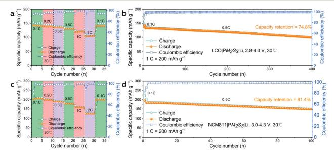
Fig. 4 Illustration of the performance metrics of the LCO $|PM_2S_3|Li$  batteries: (a) C-rate performance and (b) cycling life; and the NCM811 $|PM_2S_3|Li$  batteries: (c) C-rate performance and (d) cycling life.
