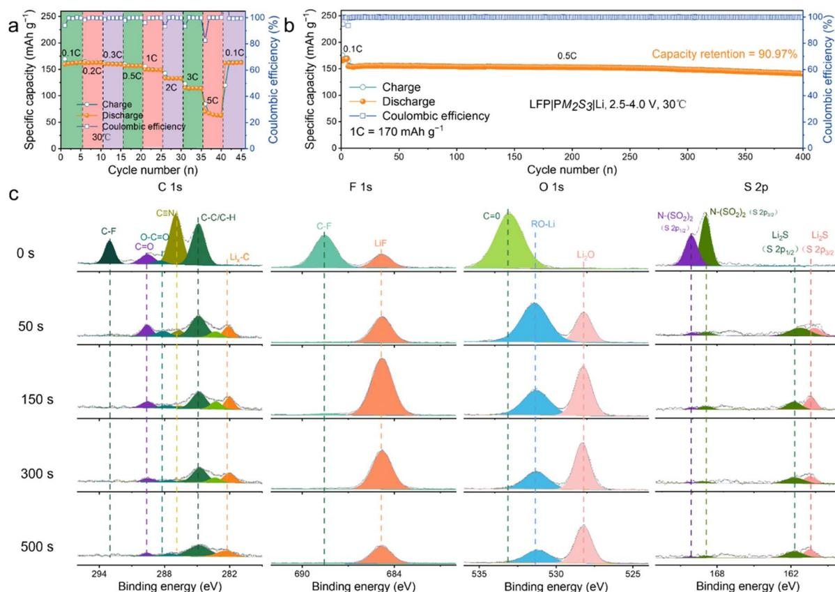
Fig. 3 Illustration of the performance metrics of the LFP|PM<sub>2</sub>S<sub>3</sub>|Li batteries: (a) C-rate performance, (b) cycling life and (c) XPS spectra for C 1s, F 1s, O 1s and S 2p core levels of the Li anode after various Ar<sup>+</sup> sputter-cleaning times. The Li anode was cycled in a Li|PM<sub>2</sub>S<sub>3</sub>|Li symmetric battery for 2000 hours.
