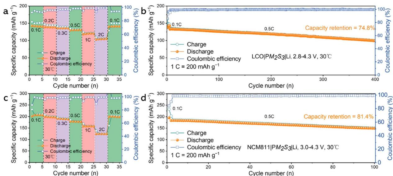
Fig. 4 Illustration of the performance metrics of the LCO|PM<sub>2</sub>S<sub>3</sub>|Li batteries: (a) C-rate performance and (b) cycling life; and the NCM811|PM<sub>2</sub>S<sub>3</sub>|Li batteries: (c) C-rate performance and (d) cycling life.
