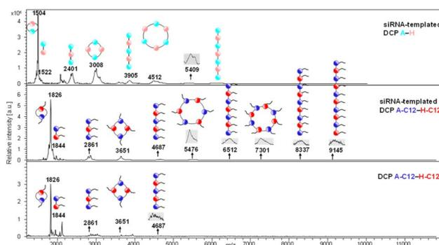
Fig. 3 MALDI-TOF characterization of DCPs. Comparative analysis of siRNA-templated (**A-H**, top; **A-C<sub>12</sub>-H-C<sub>12</sub>**, middle) and non-templated DCPs (**A-C<sub>12</sub>-H-C<sub>12</sub>**, bottom). The coloured circles represent the cationic (**A** and **H** in light blue and light red, respectively) and amphiphilic (**A-C<sub>12</sub>** and **H-C<sub>12</sub>** in blue and red) peptide monomers.
