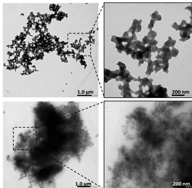
Fig. 7 TEM images of the polyplex formed *in situ* from the DCP A-C12-H-C12 (top), and of the same system in the absence of siRNA (bottom). Dynamic covalent lipopolyplexes formation was performed overnight at a monomer concentration of 1 mM in sodium acetate buffer pH 5.5.
