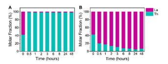
Fig. 4 Molar fractions of metals present in (A) crystalline products and (B) supernatants at specified timepoints during binary crystallization trials with an initial mixture of La( $\bowtie$ ) and Th( $\bowtie$ ) as determined by ICPOES. The time = 0 bar represents the initial concentration of metals in solution before selective crystallization. Error bars shown represent the standard deviation of three replicate trials.
