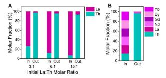
Fig. 5 Molar fractions of metals present in selective crystallization trials with (A) increased initial La: Th ratios and (B) mixture of five different trivalent REs and Th(iv). The "in" bar represents the initial concentration of metals in solution while the "out" bar represents the contents of the solid products following selective crystallization. Error bars shown represent the standard deviation of three replicate trials.
