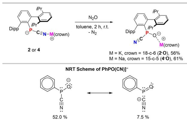
Scheme 5 Synthesis of the phosphinidene monoxide species **2·O** and **4·O** (left) and NRT scheme of the truncated model anion [PhPO(CN)]<sup>-</sup>.
