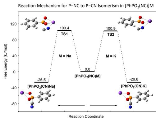
Fig. 4 Computed thermal reaction pathway for the NC/CN isomerism in model compounds  $[\text{PhPO}_2(\text{NC})]\text{M}$  ( $\text{M} = \text{Na}, \text{K}$ ) (DLPNO-CCSD(T)/def2-TZVP//PBE0-D3/def2TZVP,  $c^\circ = 1 \text{ mol L}^{-1}$ ).
