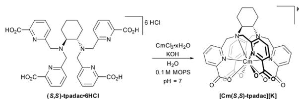
Fig. 1 Synthesis of  $[\text{Cm}(\text{S,S})\text{-tpadac}][\text{K}]$ , the other enantiomer was synthesized analogously using (*R,R*)-tpadac. MOPS: 3-(*N*-morpholino)propanesulfonic acid.
