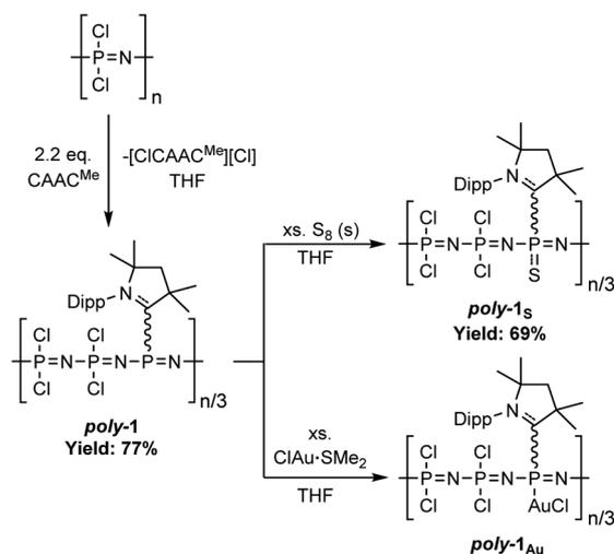
Scheme 6 Reduction of poly-chlorophosphazene to poly-**1** and its subsequent reactivity with excess S<sub>8</sub> and ClAu·SMe<sub>2</sub>. Dipp = 2,6-diisopropylphenyl.
