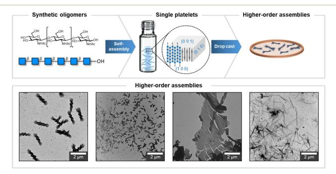
Fig. 1 The multiple levels of chitin oligosaccharides assembly. Chitin oligomers ( $N_6$ ) assemble into a colloidally stable suspension of platelets with a 3-D molecular model adopting the  $\alpha$ -chitin crystal structure. Drop casting generates different higher-order assemblies. TEM images of different types of higher-order assemblies obtained in this work. The morphologies range from defined twists, to less defined ones, to cramped material and to long, thin fibrils.
