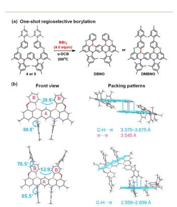
Fig. 2 (a) Synthetic route of DBNO and DMBNO. (b) Single-crystal structure of DBNO (CCDC: 2385105) and DMBNO (CCDC: 2385106).
