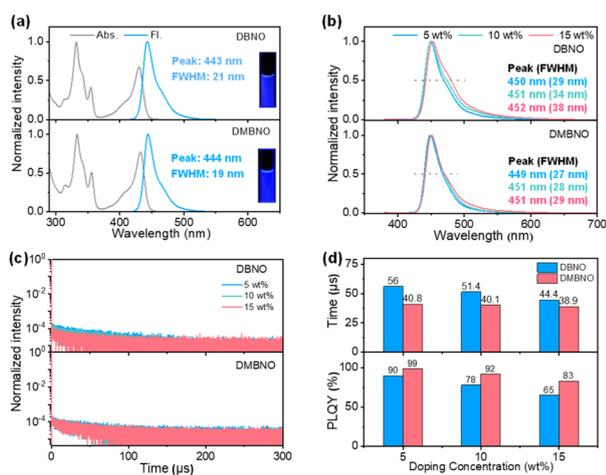
Fig. 4 Photophysical properties of **DBNO** and **DMBNO**. (a) The UV-vis spectra and fluorescence spectra in diluted toluene (inset: photographs of corresponding diluted toluene under 365 nm UV light excitation). (b) The fluorescence spectra in SiTrzCz<sub>2</sub> doped films. (c) Transient photoluminescence decay curves in SiTrzCz<sub>2</sub> doped films. (d) The delayed fluorescence ( $\tau_D$ ) lifetimes and PLQY values ( $\Phi_{PL}$ ) in SiTrzCz<sub>2</sub> doped films.
