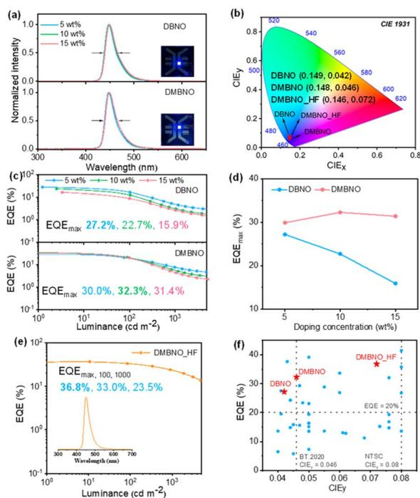
Fig. 5 (a) The EL spectra of the devices (recorded at 6 V). (b) CIE coordinates of EL emission from 5 wt% **DBNO**, 10 wt% **DMBNO** devices and HF-device of **DMBNO**. (c) EQE–luminance (EQE–L) curves of **DBNO** and **DMBNO**. (d) The EQE<sub>max</sub>–dopant concentration relationships of **DBNO** and **DMBNO**. (e) The EQE–L curve of **DMBNO** based hyperfluorescent device, inset: EL spectrum recorded at 6 V. (f) Summary of the reported MR-TADF emitters with CIE<sub>y</sub> less than 0.08.
