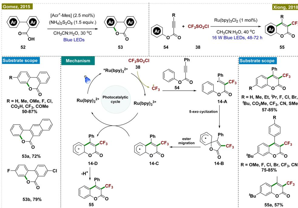
Scheme 14 Synthesis of coumarins by *ortho*-C–H cyclization.
