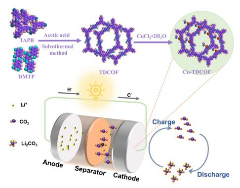
Fig. 1 Schematic synthesis of Cu-TDCOF and its use in a Li-CO<sub>2</sub> battery as a cathode catalyst.
