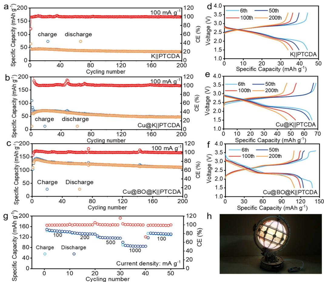
Fig. 5 Electrochemical performance of full cells. The cycling performances of (a) PTCDA||K, (b) PTCDA||Cu@K, and (c) PTCDA||Cu@BO@K full cells at  $100 \text{ mA g}^{-1}$ . Corresponding galvanostatic charge–discharge curves of (d) PTCDA||K, (e) PTCDA||Cu@K, and (f) PTCDA||Cu@BO@K full cells. (g) Rate performance of the PTCDA||Cu@BO@K full cells at different current densities of 100 to  $1000 \text{ mA g}^{-1}$ . (h) PTCDA||Cu@BO@K full cell powered LED lights.
