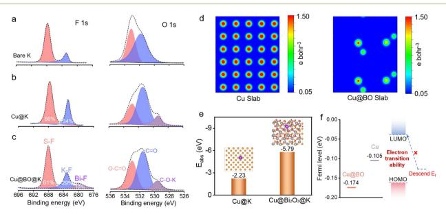
Fig. 4 XPS spectra and theoretical calculation of the hosts. High resolution F 1s and O 1s XPS of (a) bare K, (b) Cu@K and (c) Cu@BO@K host after cycles. (d) Surface charge density and (e) surface adsorption energy of Cu@K and Cu@BO@K. (f) Plots of the Fermi levels of Cu and Cu@BO host to the electrolyte.
