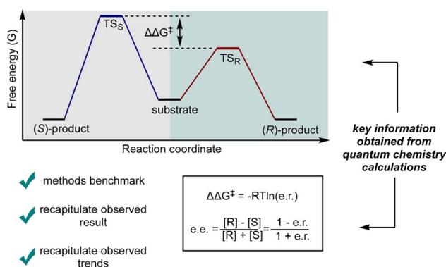
Fig. 5 Illustration of the relationship between  $\Delta\Delta G^\ddagger$  and enantioselectivity (e.r. and ee). [R] and [S] represent the concentration of R- and S-product after the reaction, respectively.
