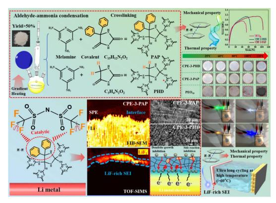
Fig. 1 Design strategy of the PAP/PHD and CPE membrane preparation process and schematic illustration of the interface stabilization mechanism.
