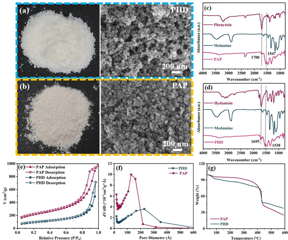
Fig. 2 Photograph and SEM image of (a) PHD and (b) PAP. FTIR spectra in the wavenumber range of 4000–800 cm<sup>-1</sup> of (c) PAP and (d) PHD. (e) Nitrogen isotherms at 298 K of PHD and PAP. (f) Pore size distribution of PHD and PAP. (g) TGA curves of PAP and PHD.
