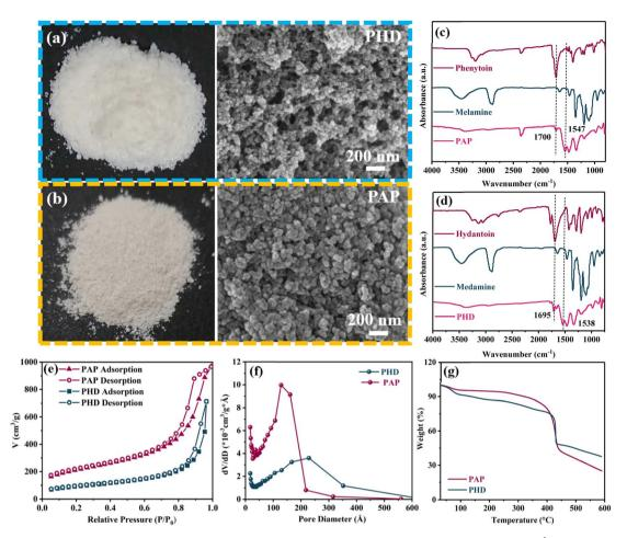
Fig. 2 Photograph and SEM image of (a) PHD and (b) PAP. FTIR spectra in the wavenumber range of  $4000-800 \text{ cm}^{-1}$  of (c) PAP and (d) PHD. (e) Nitrogen isotherms at 298 K of PHD and PAP. (f) Pore size distribution of PHD and PAP. (g) TGA curves of PAP and PHD
