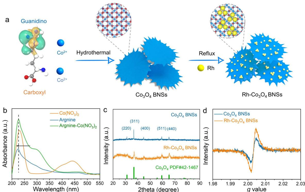
Fig. 1 (a) Schematic illustration of the preparation of Rh- $\text{Co}_3\text{O}_4$  BNSs; (b) UV-vis absorption spectra of  $\text{Co}(\text{NO}_3)_2$ , arginine and arginine- $\text{Co}(\text{NO}_3)_2$  aqueous solution; (c) XRD patterns of  $\text{Co}_3\text{O}_4$  BNSs and Rh- $\text{Co}_3\text{O}_4$  BNSs; (d) EPR spectra of  $\text{Co}_3\text{O}_4$  BNSs and Rh- $\text{Co}_3\text{O}_4$  BNSs.
