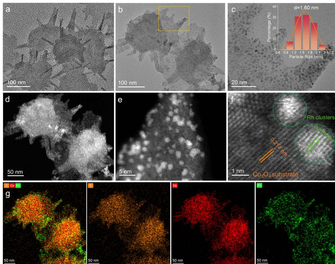
Fig. 2 (a) TEM image of  $\text{Co}_3\text{O}_4$  BNSs; (b) and (c) TEM images of Rh- $\text{Co}_3\text{O}_4$  BNSs with different resolutions, the inset of (c) shows the corresponding particle-size distribution; (d)–(f) AC-HAADF-STEM image of Rh- $\text{Co}_3\text{O}_4$  BNSs; (g) EDX element mapping images of Rh- $\text{Co}_3\text{O}_4$  BNSs.
