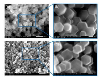
Fig. 2 (a and b) SEM images of ZIF-8 with different magnification times. (c and d) SEM images of the  $Cu_{0.5}$ @ZIF-8-MeOH precursor with different magnification times.
