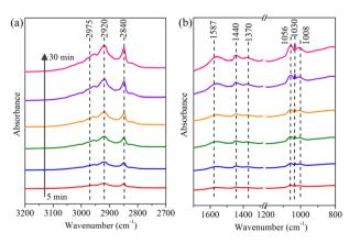
Fig. 10 In situ DRIFT spectra of  $CO_2$  hydrogenation to methanol on the CZ-0.5-R-MeOH catalyst at 220 °C and 0.1 MPa in the wavenumber range of (a) 3200-2700 cm<sup>-1</sup> and (b) 1700-800 cm<sup>-1</sup>.
