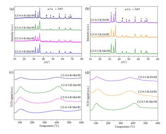
Fig. 5 (a and c) XRD patterns and CO<sub>2</sub>-TPD profiles of the reduced CZ-x-R-MeOH catalysts, where x represents the Cu/(Cu + Zn) molar ratio (x = 0.3, 0.4, 0.5, 0.6). (b and d) XRD patterns and CO<sub>2</sub>-TPD profiles of the reduced CZ-0.5-R-y catalysts, where y represents different alcohols (y = MeOH, EtOH, PrOH).
