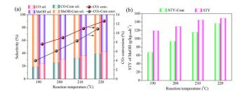
Fig. 8 (a and b) Catalytic activity comparison of the CZ-0.5-R-MeOH catalyst and the commercial Cu/ZnO catalyst at different reaction temperatures. The labels for catalytic performance of the commercial Cu/ZnO catalyst are distinguished by "Com". Reaction conditions: catalyst weight = 0.25 g, reaction pressure = 5.0 MPa, GHSV = 6000 mL  $g_{cat}^{-1} h^{-1}$ , feed gas: Ar/CO<sub>2</sub>/H<sub>2</sub> = 4/24/72.
