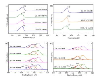
Fig. 4 (a and c)  $H_2$ -TPR profiles and O 1s XPS spectra of the calcined CZ-x-C-MeOH catalysts, where x represents the Cu/(Cu + Zn) molar ratio (x = 0.3, 0.4, 0.5, 0.6). (b and d)  $H_2$ -TPR profiles and O 1s XPS spectra of the calcined CZ-0.5-C-y catalysts, where y represents different types of alcohol (y = MeOH, EtOH, PrOH).
