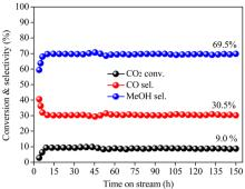
Fig. 9 Stability test of the CZ-0.5-R-MeOH catalyst for CO $_2$  hydrogenation to methanol. Reaction conditions: catalyst weight = 0.25 g, reaction temperature = 200 °C, reaction pressure = 5.0 MPa, GHSV = 6000 mL  $\rm g_{cat}^{-1} h^{-1}$ , feed gas: Ar/CO $_2$ /H $_2$  = 4/24/72.
