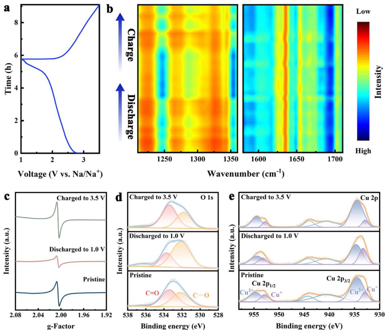
Fig. 4 (a and b) Discharge/charge profile and *in situ* FT-IR spectra of Cu-DBC. (c) *Ex situ* EPR spectra of Cu-DBC during the GCD process. (d and e) *Ex situ* XPS spectra of O 1s and Cu 2p during the GCD process.
