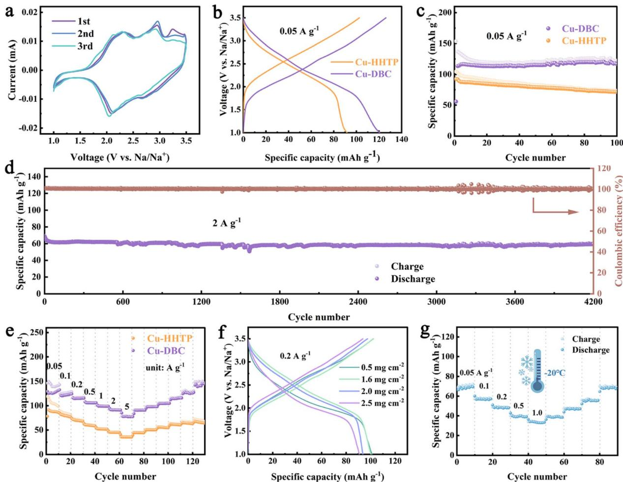
Fig. 3 (a) CV curves of Cu-DBC at  $0.1 \text{ mV s}^{-1}$ . (b) GCD profiles of Cu-DBC and Cu-HHTP at  $0.05 \text{ A g}^{-1}$ . (c) Cycling stability of Cu-DBC and Cu-HHTP at  $0.05 \text{ A g}^{-1}$ . (d) Cycling stability of Cu-DBC at  $2.0 \text{ A g}^{-1}$ . (e) Rate capability of Cu-DBC and Cu-HHTP. (f) GCD profiles of Cu-DBC at  $0.2 \text{ A g}^{-1}$  with varying active mass loading. (g) Rate capability of Cu-DBC at  $-20^\circ\text{C}$ .
