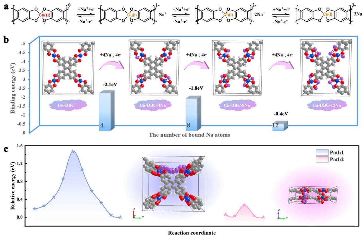
Fig. 5 (a) Schematic of the  $\text{Na}^+$  storage process in the  $[\text{CuO}_4]$  units. (b)  $\text{Na}^+$  storage behaviour of Cu-DBC. (c)  $\text{Na}^+$  migration pathways and associated energy barrier.
