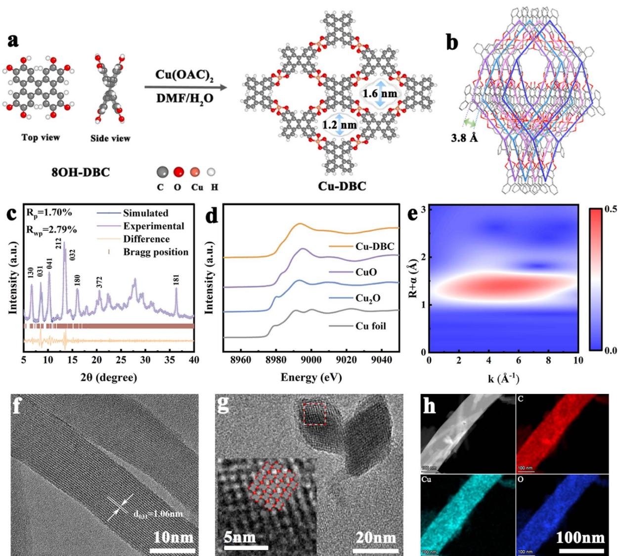
Fig. 2 (a) Synthetic diagram of Cu-DBC. (b) Topological structure of Cu-DBC. (c) PXRD patterns. (d) Cu K-edge XANES spectra of Cu-DBC, Cu foil, Cu<sub>2</sub>O, and CuO. (e) Wavelet transform-EXAFS signals of Cu-DBC. (f and g) HRTEM images of Cu-DBC. (h) HAADF-STEM mappings of the elements Cu, O, and C for Cu-DBC.
