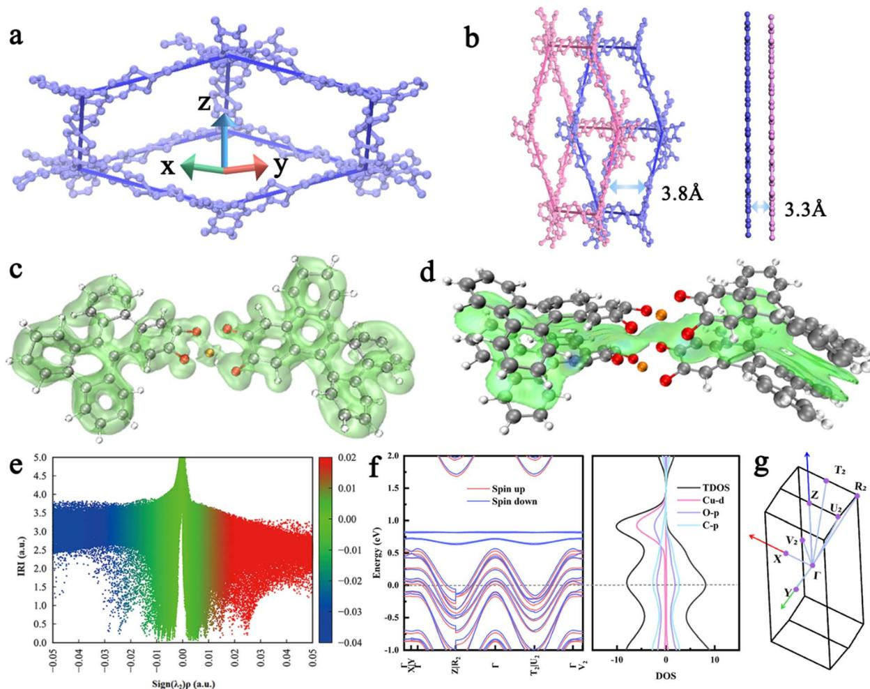
**Fig. 1** (a) Diagram of Cu-DBC in one-fold interpenetration. (b) Diagram of double interpenetration for Cu-DBC and double layers for Cu-HHTP. (c) LOL- $\pi$  isosurface of Cu-DBC segments. (d)  $\text{Sign}(\lambda_2)\rho$  of Cu-DBC corresponding to IGMH analyses. (e) Colored scatter map between IRI and  $\text{sign}(\lambda_2)\rho$ . (f) Electronic band structure and density of states (DOS) of Cu-DBC. (g) The Brillouin zone of the Cu-DBC unit cell.
