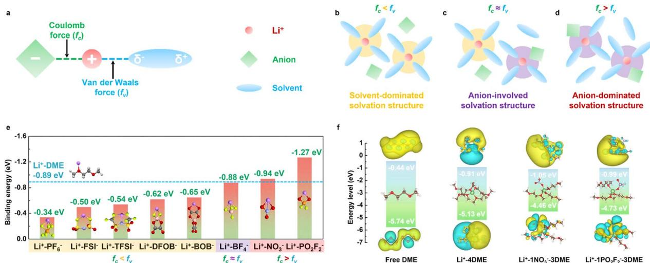
Fig. 1 (a) Schematic diagram of the microscopic forces between Li<sup>+</sup>, anions and solvent molecules. (b–d) Schematic diagram of different types of solvation structures. (b) Conventional electrolyte, (c) WSE, and (d) SCE. (e) Comparison of the binding energy of Li<sup>+</sup> with DME molecules and different anions. (f) Comparison of LUMO–HOMO energy levels of typical solvation structures.
