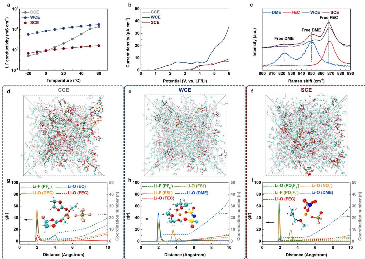
Fig. 2 (a) The  $\text{Li}^+$  conductivity comparison of studied electrolytes at various temperatures. (b) LSV plots of studied electrolytes. (c) Locally amplified Raman spectra for different solutions. (d–f) Snapshots of the MD simulation cell and (g–i) the corresponding radial distribution functions of different electrolytes: (d) and (g) CCE, (e) and (h) WCE, (f) and (i) SCE. The insets show the representative  $\text{Li}^+$  solvation structures of the electrolytes.
