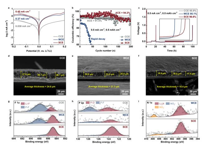
Fig. 3 (a) Tafel plots of Li-Li symmetric cells using studied electrolytes. Li-Cu half-cell (b) cycling and (c) CE tests using different electrolytes (test conditions: 0.5 mA cm<sup>-2</sup>, 0.5 mA h cm<sup>-2</sup> for 20 cycles). SEM cross-sectional images of deposited Li using (d) CCE, (e) WCE, and (f) SCE (deposition conditions:  $0.5 \text{ mA cm}^{-2}$  for  $3 \text{ mA h cm}^{-2}$ ). (g) XPS F 1s, (h) P 2p, and (i) N 1s spectra of metallic Li deposited from different electrolytes.
