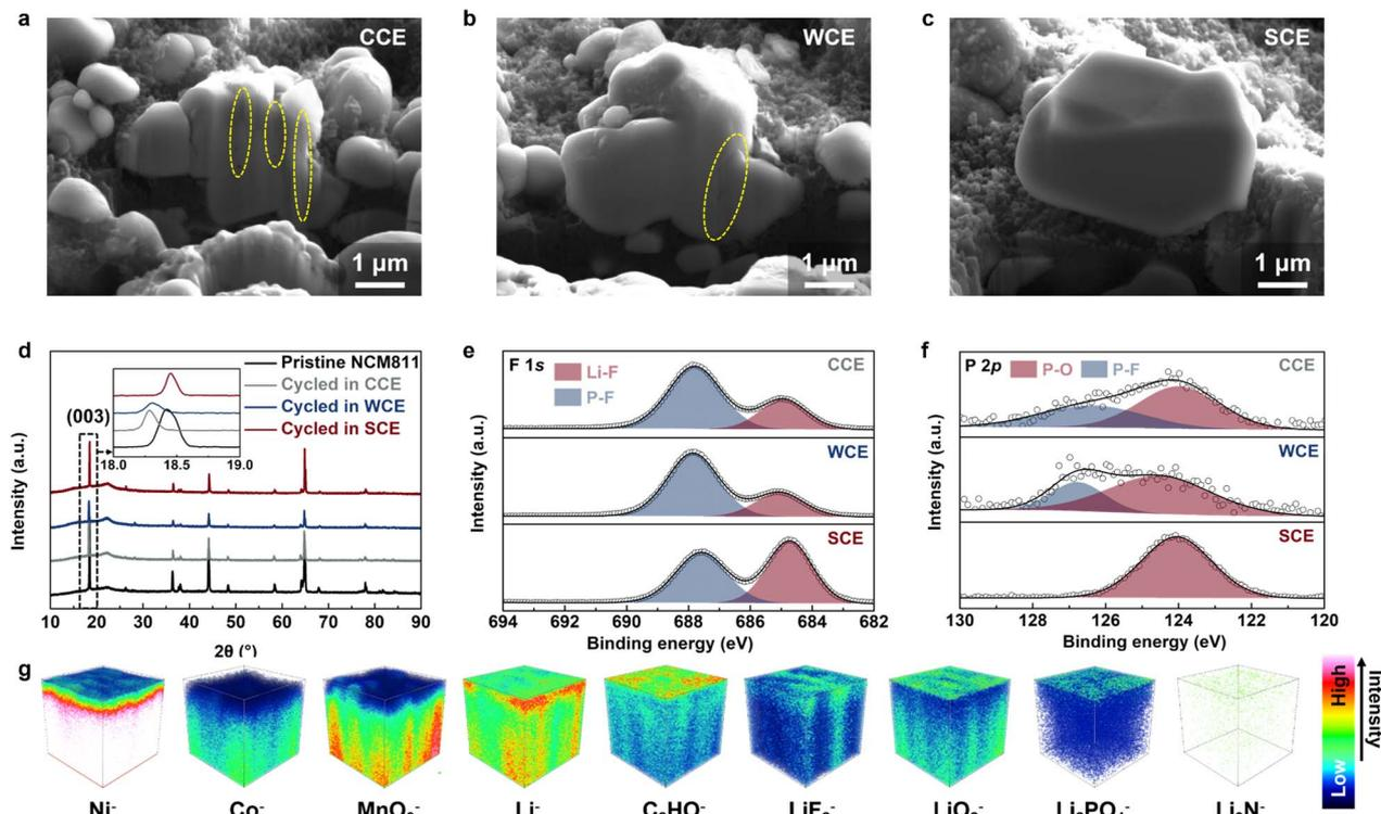
Fig. 5 FIB-SEM images of cycled NCM811 cathodes using different electrolytes: (a) CCE, (b) WCE, (c) SCE. (d) XRD patterns of pristine and cycled NCM811 cathodes in the studied electrolytes. The inset shows a locally amplified XRD pattern. (e) The F 1s spectra and (f) P 2p spectra comparison of the cycled NCM811 cathodes in different electrolytes. (g) 3D views of the CEI composition detected by TOF-SIMS depth sputtering on the surface of cycled NCM811 using SCE.
