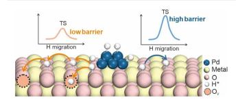
Fig. 8 Mechanism of oxygen vacancies affecting hydrogen spillover.
