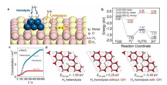
Fig. 5 (a) Mechanism of oxygen vacancies affecting hydrogen dissociation. (b) Calculated energy profiles of adsorption and dissociation of H<sub>2</sub>. Reproduced from ref. 30. Copyright 2022 Springer Nature. (c) The evolution of surface Ga-H and Ga-OH over α-Ga<sub>2</sub>O<sub>3</sub> samples with contact time of  $H_2$  at 350 °C. (d)  $H_2$  adsorption energy by homolytic dissociation over  $\alpha$ - $Ga_2O_3$  (001). Reproduced from ref. 29. Copyright 2024 Springer
