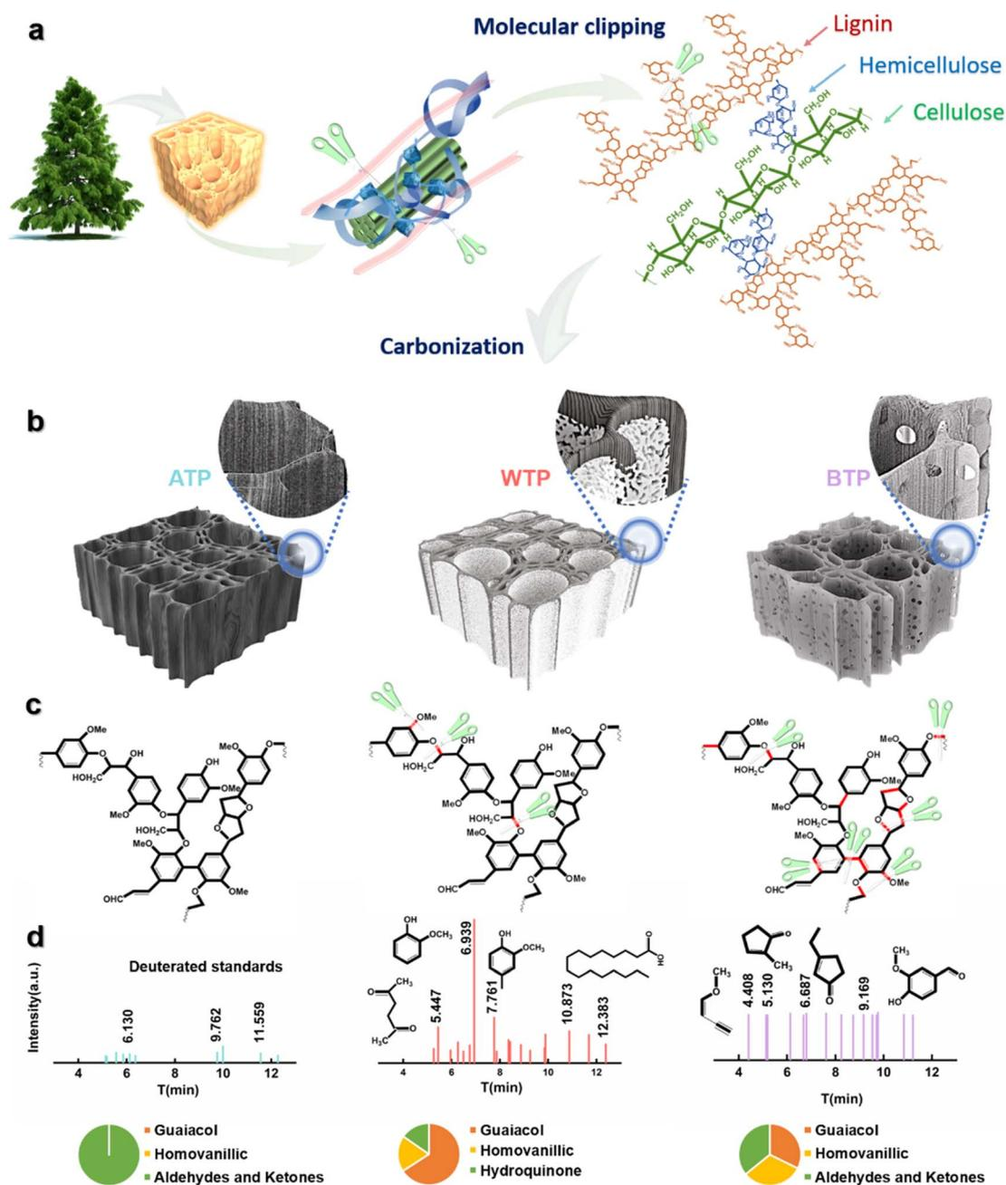
**Scheme 1** The formation process of carbon frameworks derived from biomass wood and the bond cleavage of lignin in wood. (a and b) Schematic illustration of the fabrication and the structures of ATP, WTP and BTP. (c) Cleavage location of lignin bonds in ATP, WTP and BTP. (d) GC-MS analysis of the solution after the hydrothermal reaction of ATP, WTP and BTP (pie chart illustrates the content of the pyrolysis product).
