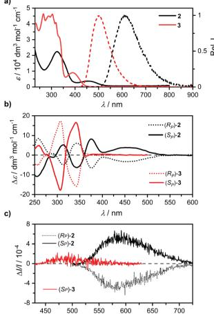
Fig. 2 (a) UV-Vis absorption (solid line) and fluorescence (dashed line) spectra of 2 and 3. (b) ECD of 2 and 3 ( $\Delta \varepsilon$  of 3 scaled by 0.1) and (c) CPL spectra of 2 and 3. All samples were measured in dichloromethane (c  $\sim 5 \times 10^{-5} \text{ M}$
