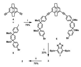
Scheme 1 Synthesis of BT containing macrocycles 2 and 3. Reaction conditions: (i)  $Pd_2dba_3$ ,  $PPh_3$ , Cul, THF/TEA, RT, 4 h. (ii)  $K_3PO_4$ , SPhos Pd Gen 3, dioxane, 80 °C, 18 h (iii) A:  $SnCl_2$ , HCl, THF, RT, 2 h or B: Na, Na
