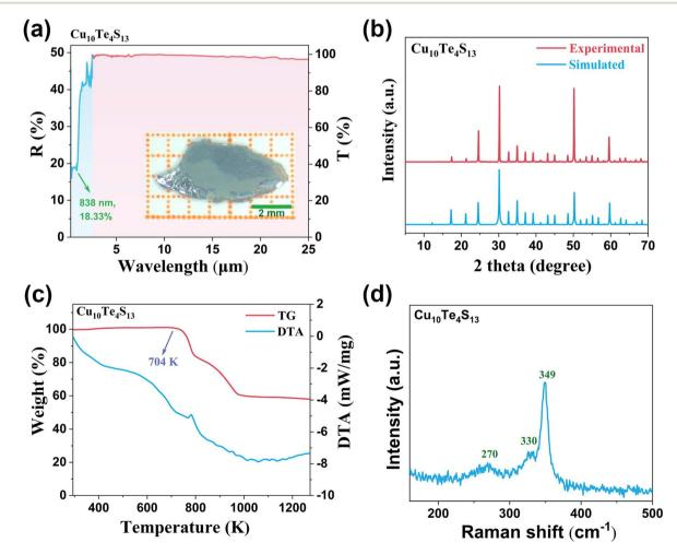
Fig. 3 (a) The UV-vis-IR spectrum of  $Cu_{10}Te_4S_{13}$  and the inset shows a photo of a large polished crystal of  $Cu_{10}Te_4S_{13}$ . (b) simulated and experimental powder X-ray diffraction patterns of  $Cu_{10}Te_4S_{13}$ ; (c) TG-DTA of  $Cu_{10}Te_4S_{13}$  under a  $N_2$  atmosphere; (d) Raman spectrum of  $Cu_{10}Te_4S_{13}$ .
