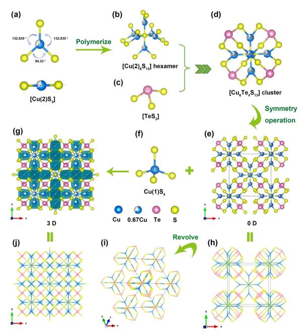
Fig. 1 (a) Planar triangular  $[Cu(2)S_3]$  motif; (b) unique  $[Cu_6S_{13}]$  hexamer; (c)  $[TeS_3]$  triangular pyramid; (d) butterfly-orchid-like  $[Cu_6Te_4S_{13}]^{4-}$  0D anion cluster; (e) [Cu(2)-Te-S] 0D framework; (f)  $[Cu(1)S_4]$  tetrahedron; (g) the 3D structure of  $Cu_{10}Te_4S_{13}$ ; (h and i) the wireframe of the 0D framework; (j) the wireframe of the 3D structure.
