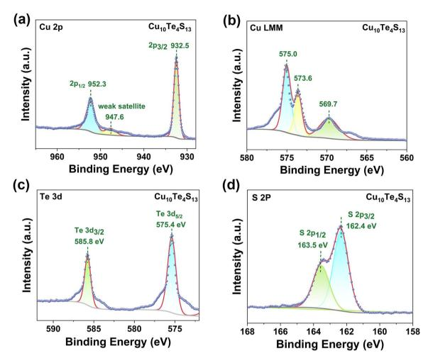
Fig. 2 (a) Cu 2p XP spectrum; (b) Cu LMM auger XP spectrum; (c) Te 3d XP spectrum; (d) S 2p XP spectrum of Cu<sub>10</sub>Te<sub>4</sub>S<sub>13</sub>.
