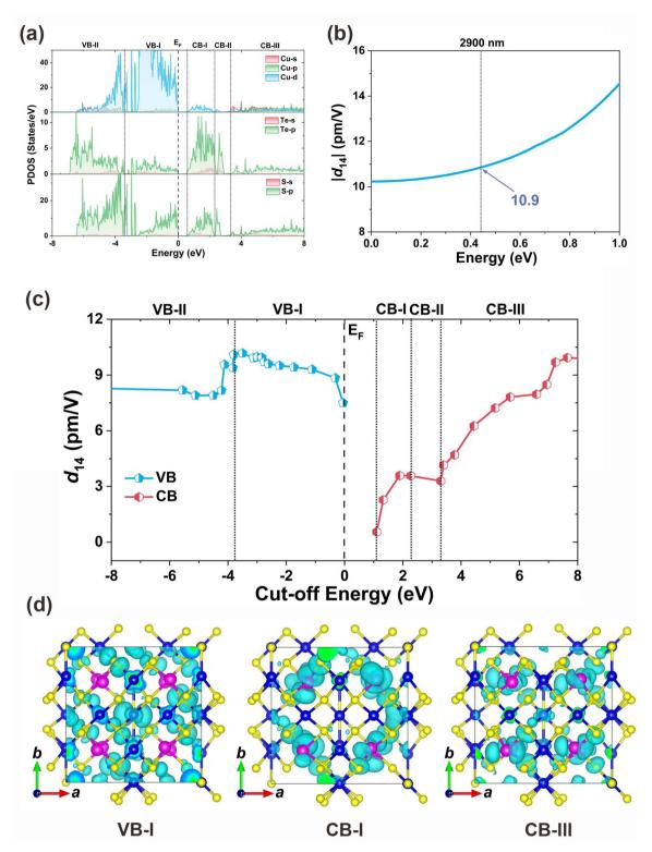
Fig. 5 Theoretical calculations of  $Cu_{10}Te_4S_{13}$ : (a) PDOS diagrams projected onto constituent atoms; (b) frequency-dependent SHG tensor  $d_{14}$ ; (c) relationship between SHG tensor  $d_{14}$  (pm  $V^{-1}$ ) and cut-off energy (eV); (d) partial charge density distribution diagrams showing the main contributions of VB-I, CB-I and CB-III regions. Blue atoms represent Cu, pink atoms represent Te, and yellow atoms represent S.
