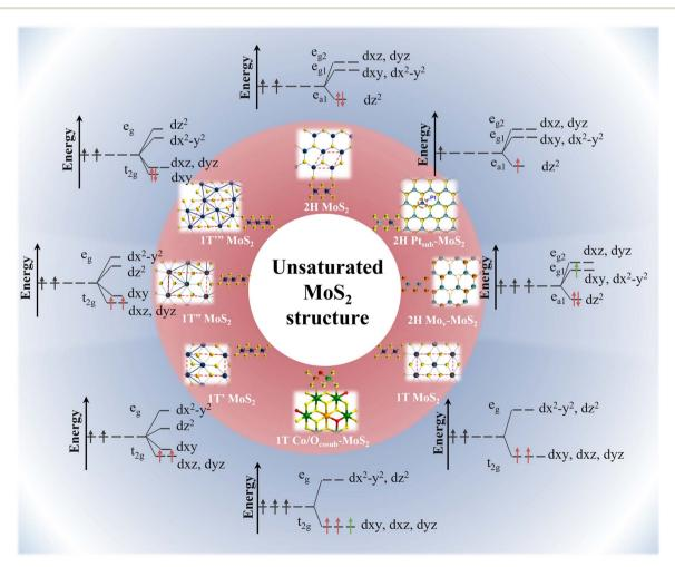
Fig. 3 Orbital electron unsaturation strategy for MoS<sub>2</sub> electrocatalysts based on crystal field theory.
