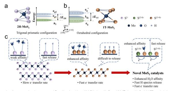
Fig. 2 The unit cell structure, band structure and Fermi level position of (a) 2H phase MoS<sub>2</sub> and (b) 1T phase MoS<sub>2</sub>. (c) HER catalytic behavior on 2H phase MoS<sub>2</sub>, 1T phase MoS<sub>2</sub>, and the principle to modify MoS<sub>2</sub>.
