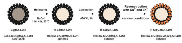
Fig. 1 Synthetic scheme used to obtain mixed-metal (Cu, Zn) hollow-SiO<sub>2</sub>@Cu<sub>2</sub>Zn<sub>1</sub>Mq<sub>2</sub>Al-LDH spheres.
