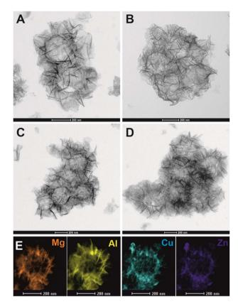
Fig. 4 TEM images of H-S@CZMA-LDHs obtained after immersing H-S@MA-LDO in solutions containing  $Cu^{2+} + Zn^{2+}$  at a concentration of 20 mM (A), 40 mM (B), 60 mM (C) and 80 mM (D) and Mg, Al, Cu, Zn elemental EDX mapping of H-S@CZMA-LDH\_20 mM (E).
