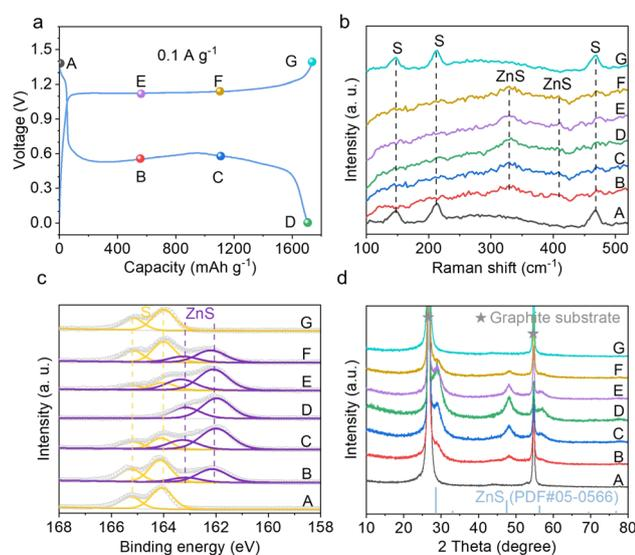
Fig. 4 (a) Charge-discharge curves of the Zn-S cell in the Br<sup>-</sup> containing electrolyte at 0.1 A g<sup>-1</sup>, and the corresponding (b) Raman spectra, (c) fitted S 2p XPS and (d) XRD patterns of the cathode at the labelled states.
