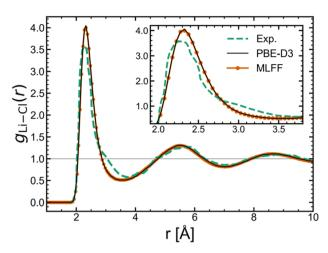
Fig. 1 Comparison of the Li–Cl radial distribution function between experiment,<sup>32</sup> DFT, and MLFF.
