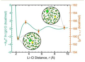
Fig. 3 Dual-axis plot of the potential of mean force between  $Li^+$  and  $Cl^-$  based on g(r) (left axis, solid green line) and the excess chemical potential computed at multiple fixed Li-Cl distances (right axis, orange markers). Insets show representative configurations at the corresponding Li-Cl distance with the targeted ions highlighted. System conditions for each calculation match those in Fig. 2.
