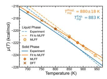
Fig. 5 Solid and liquid phase chemical potentials from MLFF and DFT predictions compared to experiment.<sup>45</sup> Uncertainties of the fitted lines are omitted for clarity, but error bars of MLFF and DFT data points are smaller than the size of the markers.
