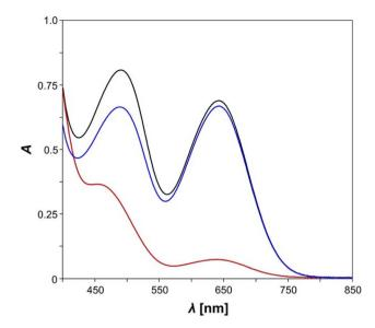
Fig. 2 UV/vis spectra of *E*-5B before (black line), directly after irradiation with light (red line) and after 30 minutes in the dark, *i.e.*, after the thermal reverse reaction (blue line), c = 0.14 mmol L<sup>-1</sup>, benzene.
