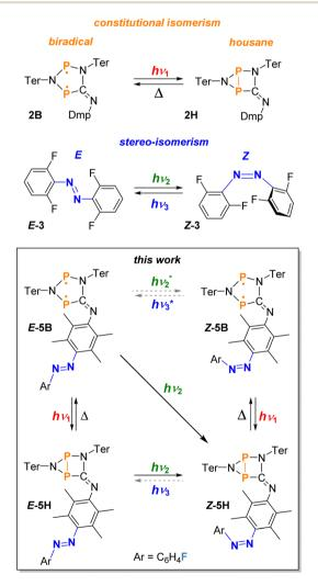
Scheme 1 Examples of molecular switches undergoing either constitutional or stereo-isomerisation upon irradiation with visible light (top) and the combination of these types of switches to a novel visible light-mediated double photoswitch as part of this work (bottom). Reactions indicated by asterisks are presumed to take place under irradiation but cannot be traced spectroscopically as always housane formation occurs.<sup>35,49</sup>
