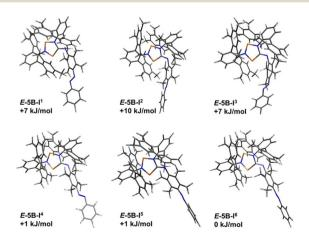
Fig. 8 Graphical representation of the significant calculated isomers of *E*-5B, which were identified as the six lowest lying isomers (standard Gibbs free energies in relation to the lowest energy isomer).
