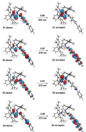
Fig. 7 Natural transition orbitals (NTOs) of *E*-5B. States S1 to S4 (with contributing coefficients) are depicted alongside the corresponding wavelengths.
