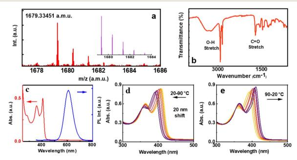
Fig. 2 (a) MALDI-TOF and (b) FT-IR spectra of MUA capped Au clusters. Inset in 'a' shows the simulated mass spectrum. (c) Absorption (red trace) and emission (blue trace) spectra of the clusters in water. Absorption spectral changes during (d) gradual heating of clusters to 90 °C and (e) upon cooling back to room temperature.
