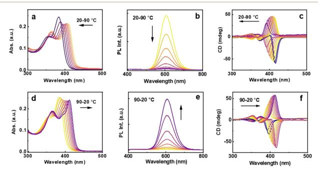
Fig. 5 (a) and (d) UV-visible, (b) and (e) luminescence and (c) and (f) CD spectral responses with (a) – (c) a gradual increase in temperature from 20 °C to 90 °C, and (d)-(f) upon cooling back to 20 °C.
