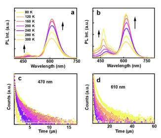
Fig. 4 Temperature dependent PL spectra of MUA capped Au<sub>4</sub> clusters in the (a) absence and (b) presence of the chiral surfactant DMEB. Temperature dependent lifetime plot of MUA capped Au<sub>4</sub> clusters in the presence of DMEB for emission monitored at (c) 470 nm and (d) 610 nm.
