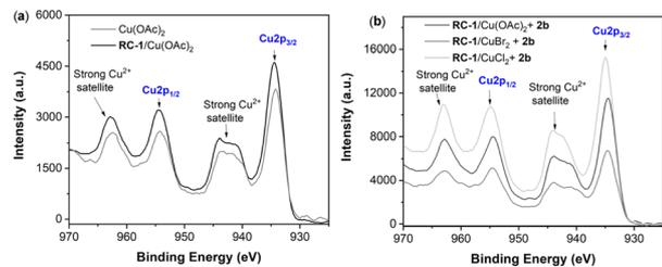
Fig. 1 XPS analysis. (a) Comparison of Cu(OAc)<sub>2</sub> and RC-1/Cu(OAc)<sub>2</sub>. (b) XPS of RC-1 with different copper salts after adding the substrate of 3-oxopentanoic acid (2b).
