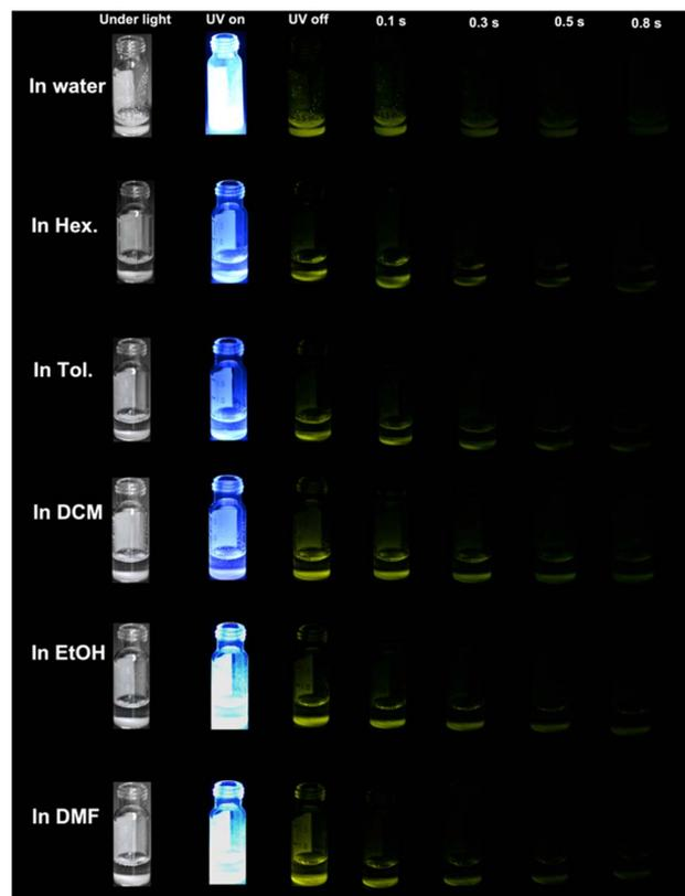
Fig. 4 The photographs of single crystals of **CityU-21** immersed in different solvents with RTP properties.
