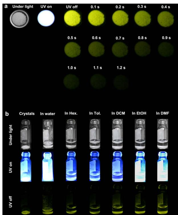
Fig. 3 (a) The photographs of single crystals of **CityU-21** before and after switching off 365 nm UV light. (b) The photographs of single crystals of **CityU-21** treated with/without solvents before and after switching off 365 nm UV light.
