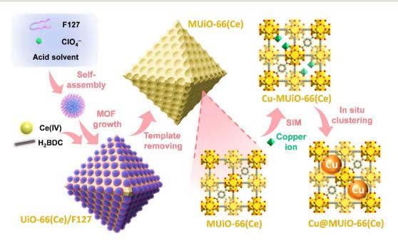
Fig. 1 Schematic illustration of the synthetic process for preparing MUiO-66(Ce), Cu-MUiO-66(Ce), and Cu@MUiO-66(Ce). Yellow, red, and gray atoms shown in crystal structures represent Ce, O, and C, respectively. Hydrogen atoms are not shown for clarity.
