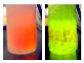
Fig. 7 Fluorescence of the vials containing  $CH_2Cl_2$  solutions of *trans*-1-O at 77 K (liquid  $N_2$ ) (left) and 2 minutes after being taken out of the liquid  $N_2$  (right).
