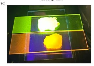
Fig. 6 Emission spectra of the PMMA films containing (a) 0.2 wt% and (b) 1.2 wt% of the benzo-fused series 1. (c) Emission color of the PMMA films with 0.2 wt% (top), and 1.2 wt% (bottom) trans-1-O.
