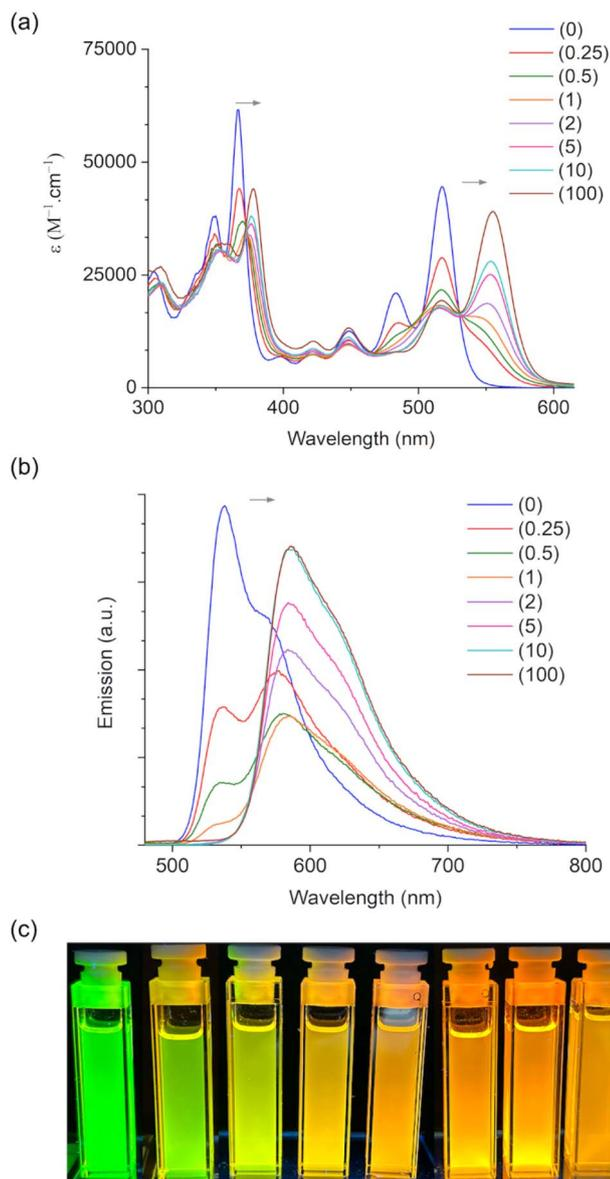
Fig. 8 Absorption (a) and emission (b) spectra of *cis-2-O* upon titration with BCF in  $\text{CH}_2\text{Cl}_2$ . (c) Solutions with equal concentrations of *cis-2-O* with increasing amounts of BCF from 0 (left) to 100 (right) equivalents.
