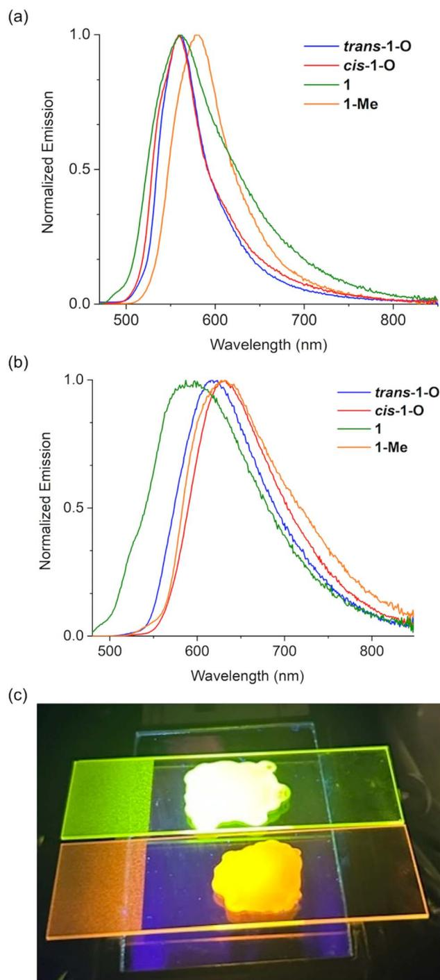
Fig. 6 Emission spectra of the PMMA films containing (a) 0.2 wt% and (b) 1.2 wt% of the benzo-fused series **1**. (c) Emission color of the PMMA films with 0.2 wt% (top), and 1.2 wt% (bottom) *trans*-1-O.
