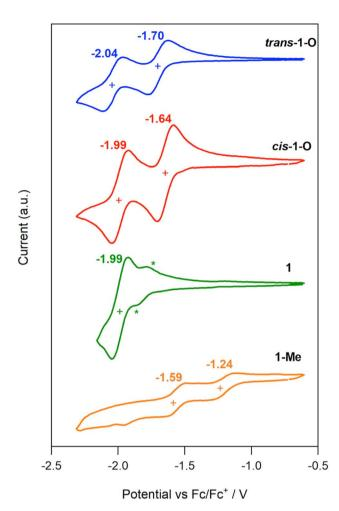
Fig. 9 Cyclic voltammograms of *trans-*1-O (blue), *cis-*1-O (red), 1 (green; \* indicate the anodic and cathodic redox processes for the second isomer), 1-Me (orange), with scan rate 100 mV s<sup>-1</sup>, in  $CH_2Cl_2$  with 0.1 M  $NBu_4PF_6$ , vs.  $Fc/Fc^+$ .
