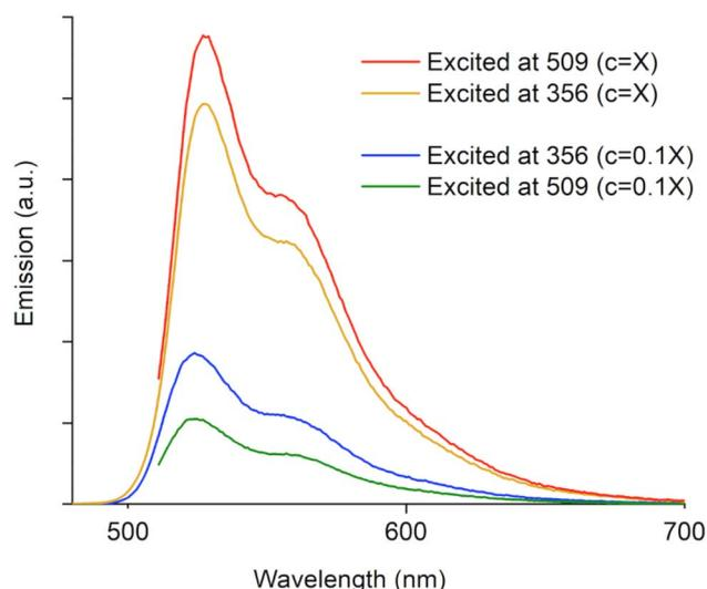
Fig. 5 Concentration-dependant emission spectra of *trans*-1-O excited at 356 and 509 nm in CH<sub>2</sub>Cl<sub>2</sub> ( $X = 6.4 \times 10^{-6}$  M).
