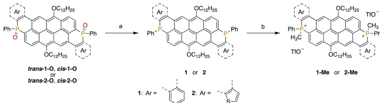
Scheme 2 P-modification reactions of **1-O** and **2-O** toward **1** and **2** and further modification toward **1-Me** and **2-Me**, both as mixtures of isomers (inseparable); (a)  $\text{HSiCl}_3$ , THF, MW, 150 °C, 20 min. (b) MeOTf,  $\text{CH}_2\text{Cl}_2$ , 0 °C  $\rightarrow$  RT, 12 h.
