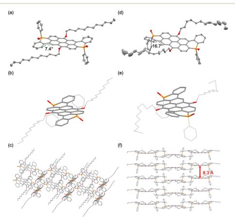
Fig. 2 Solid-state structures obtained by crystallization from toluene of trans-1-O: (a) single molecule, (b) molecular curvature, (c) packing; and cis-1-O (d) single molecule (one enantiomer shown), (e) molecular curvature, (f) packing ((a and d) 50% probability level, H-atoms omitted for clarity).
