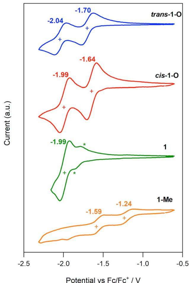
Fig. 9 Cyclic voltammograms of *trans-1-O* (blue), *cis-1-O* (red), **1** (green; \* indicate the anodic and cathodic redox processes for the second isomer), **1-Me** (orange), with scan rate  $100 \text{ mV s}^{-1}$ , in  $\text{CH}_2\text{Cl}_2$  with  $0.1 \text{ M NBu}_4\text{PF}_6$ , vs.  $\text{Fc/Fc}^+$ .
