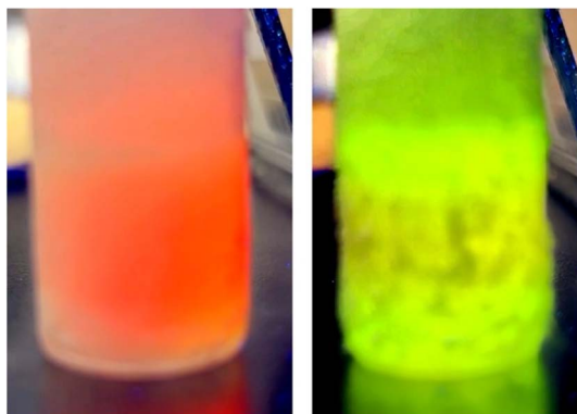
Fig. 7 Fluorescence of the vials containing \text{CH}_2\text{Cl}_2 solutions of trans -1-O at 77 K (liquid \text{N}_2 ) (left) and 2 minutes after being taken out of the liquid \text{N}_2 (right).
