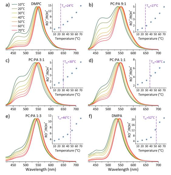
Fig. 2 Normalized temperature-dependent steady-state fluorescence measurements of C<sub>12</sub>-HPTS within membranes composed of (a) DMPC, DMPC: DMPA ratios of (b) 9:1, (c) 3:1, (d) 1:1, (e) 1:3, and (f) DMPA. The insets show the RO\*/ROH\* as a function of temperature.
