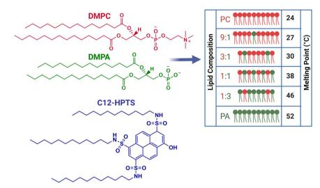
Fig. 1 Molecular structures of the DMPC and DMPA lipids and the ratios of these lipids used for making six different vesicles together with the molecular structure of  $C_{12}$ -HPTS. The melting points of different lipid membranes were measured using differential scanning calorimetry experiments.
