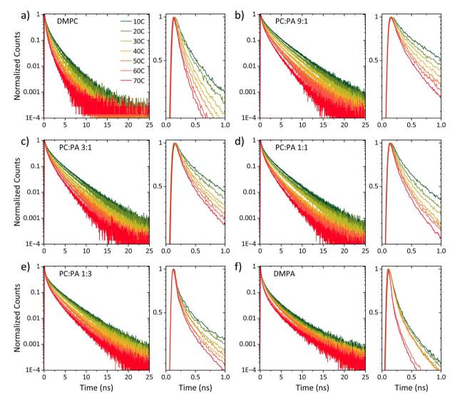
Fig. 3 Normalized temperature-dependent time-resolved fluorescence measurements of  $C_{12}$ -HPTS within membranes composed of (a) DMPC, DMPC : DMPA ratios of (b) 9:1, (c) 3:1, (d) 1:1, (e) 1:3, and (f) DMPA. The right panels zoom in on the first nanosecond of the decay.
