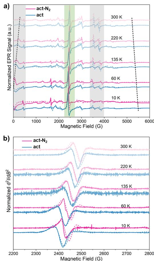
Fig. 6 (a) CW EPR spectra of **La-Gd-LOF1\_act** and **La-Gd-LOF1\_act-N<sub>2</sub>** at different temperatures. The green and grey areas highlight the differences between both spectra. (b) Second derivatives of the EPR signals at the green region previously selected. Dashed lines represent simulated spectra.
