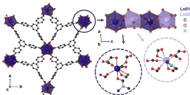
Fig. 1 (Left) Crystal structure of LOF1. Hydrogen atoms and solvent molecules have been omitted for clarity. (Top right) Rodlike chains that run parallel to the *c*-axis. The two crystallographically different lanthanoid atoms are depicted in dark and light purple. (Bottom right) Coordination environment of the lanthanoid centres. More details can be found in Fig. S2 and S3.†
