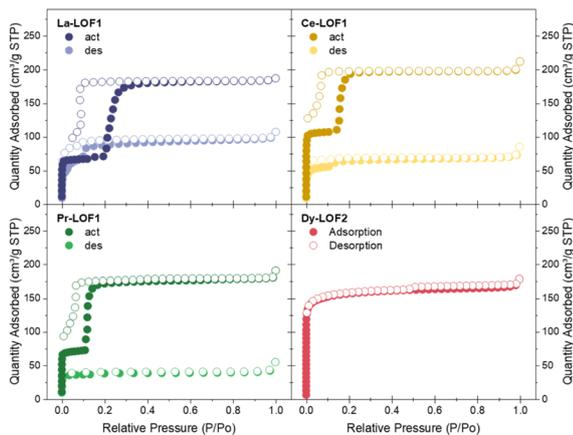
Fig. 3 N<sub>2</sub> adsorption isotherms of La-LOF1 (blue), Ce-LOF1 (yellow), Pr-LOF1 (green), and Dy-LOF2 (red) at 77 K. For La, Ce, and Pr-LOF1, activated and desolvated forms were measured and are depicted in darker and lighter colours, respectively.
