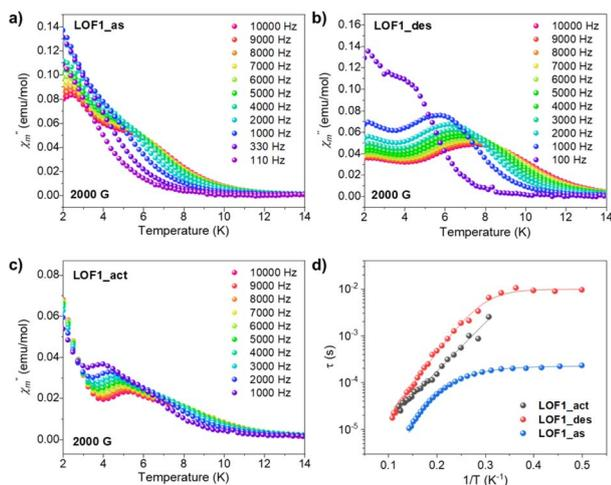
Fig. 4 Temperature dependence of the out-of-phase signal  $\chi''$  of La-Dy-LOF1\_as (a), La-Dy-LOF1\_des (b) and La-Dy-LOF1\_act (c) at different frequencies, under 2000 G DC magnetic fields. (d) Comparison of the temperature dependence of relaxation times of the three samples at 2000 G applied DC field. Solid lines represent the fitting including Orbach, Raman and quantum tunnelling of magnetisation (see the text<sup>†</sup>).
