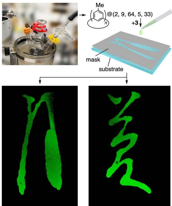
Fig. 5 Processes and images of screen-printed OLEDs using the raw-material mixture of methylated  $[n]$ CMPs from  $(M, T, C, R, S) = (2, 9, 64, 5, 33)$ . The screen-printed images were created by copying kanji characters ((left): moon, (right): dream) written by a Japanese poet, Basho Matsuo.<sup>20</sup>
