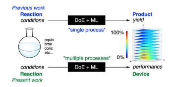
Fig. 1 "DoE + ML" method. Optimisation of reaction conditions traditionally correlates the conditions with the yields, but the present work demonstrates that the optimisation can correlate the reaction conditions with the performances of organic devices obtained through multistep processes.
