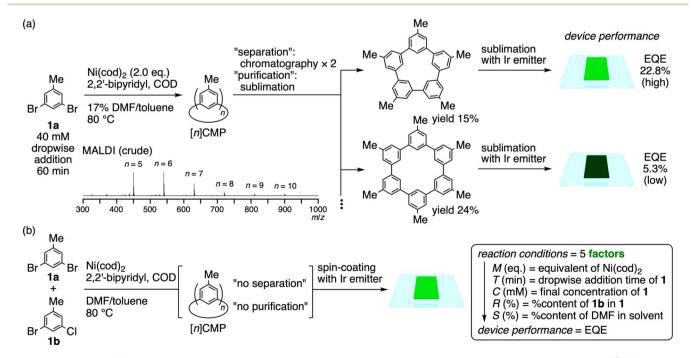
Fig. 2 Fabrication of [n]CMP-based OLEDs. (a) Multistep, stepwise processes used in traditional device fabrication protocols. (b) Simplified multistep processes used in the present study, which eliminated energy-consuming and waste-producing separation and purification steps.
