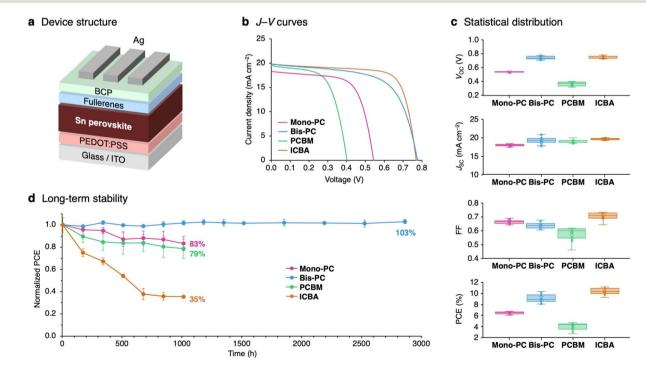
Fig. 3 Comparison of fullerene-based electron-transporting materials. (a) Device structure and (b) current-voltage (J-V) curves of tin perovskite solar cells using different electron-transporting materials. (c) Statistical distribution of photovoltaic parameters and (d) long-term stability under nitrogen conditions
