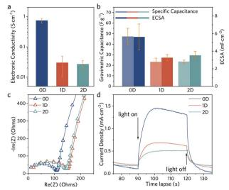
Fig. 4 (a) Electrical conductivity of 0D, 1D, and 2D Cu-HHTP. (b) Bar graph showing the gravimetric capacitance (light colors) and ECSA (dark colors) of 0D, 1D, and 2D Cu-HHTP. (c) EIS and (d) transient photocurrent response of 0D, 1D, and 2D Cu-HHTP.
