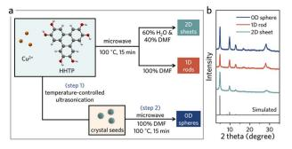
Fig. 1 (a) Schematic of the synthesis of OD, 1D, and 2D Cu-HHTP based on microwave and temperature-controlled ultrasonication treatment. (b) PXRD patterns of 0D, 1D, and 2D from the respective synthetic methods. The gray line indicates the simulated PXRD pattern.
