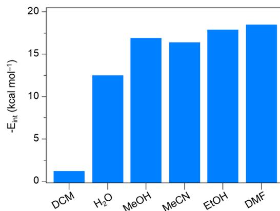
Fig. 3 DFT-calculated interaction energies for the coordination of various solvent molecules at Cu(II) OMS per unit cell of HKUST-1, indicating the coordination strength.
