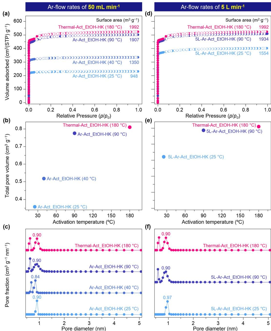
Fig. 5 (a and d)  $N_2$  adsorption/desorption isotherms, (b and e) plot of total pore volume as a function of activation temperature, and (c and f) NLDFT calculation for the pore size distribution of EtOH-HKUST-1 under different activation conditions: thermal activation at 180 °C (pink), Ar activation at 90 °C (dark blue), Ar activation at 40 °C (blue), and Ar activation at 25 °C (light blue) after (a–c) 50 mL min<sup>-1</sup> and (d–f) 5 L min<sup>-1</sup> Ar-flow activation.
