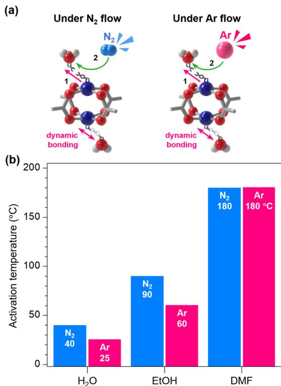
Fig. 4 (a) Schematic illustrations of the dynamic coordination bonding of H<sub>2</sub>O molecule and its dissociation process under N<sub>2</sub> (left) and Ar flow (right) conditions. (b) Activation temperatures of H<sub>2</sub>O-, EtOH-, and DMF-coordinated to HKUST-1 under N<sub>2</sub> (blue columns) and Ar (pink columns) flow conditions, showing the impact of different inert gases on the activation temperature.
