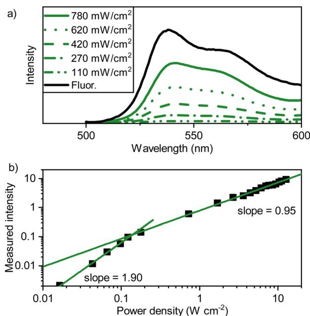
Fig. 4 (a) Emission spectra of a PdTNP-tetracene film (evaporated; 500 nm on quartz, 1% PdTNP, green lines) with incident power of the laser beam indicated ( $\lambda_{\text{exc}} = 690 \text{ nm}$ , CW,  $\varnothing = 2 \text{ mm}$ ). In black the conventional fluorescence spectrum ( $\lambda_{\text{exc}} = 475 \text{ nm}$ ) of a neat tetracene film is shown, (b) power density dependence of the PdTNP-tetracene thin film emission, excited at 690 nm.
