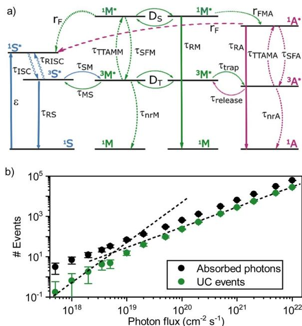
Fig. 6 (a) Scheme of the rates used in the Monte-Carlo simulations. The values of rates are given in Table S1.† (b) Emission events as a function of the incident photon flux for a system of 1% sensitizers in a host matrix (tetracene). The two dashed lines have a slope of 1 and 2 as visual guides.
