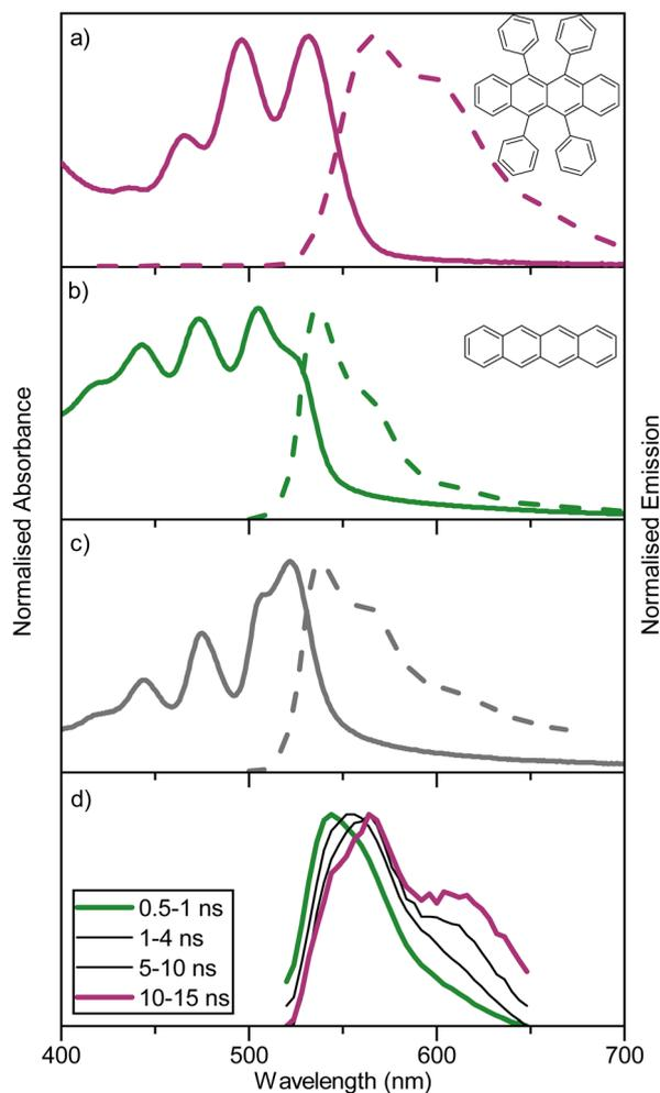
Fig. 2 Absorption and steady-state emission spectra for evaporated films of (a) rubrene, (b) tetracene, and (c) 5% rubrene in tetracene ( $l_{\text{exc}} = 475$  nm), taken as 100 nm thin films on quartz substrates fabricated through thermal evaporation. (d) Normalised TRES spectra of a thermally evaporated film (100 nm thickness on quartz) containing 5 vol% rubrene in tetracene, integration times after the excitation pulse are indicated.
