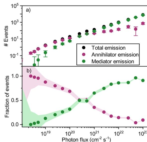
Fig. 7 (a) Simulated emission events resulting in emission in a ternary blend with 1% sensitizers and 0.1% of annihilators in a host (mol mol<sup>-1</sup>). (b) Simulated fraction of upconversion events due to hetero-TTA (purple) and homo-TTA (green).
