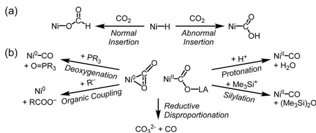
Scheme 4 (a) Normal and abnormal insertion of CO<sub>2</sub> into nickel hydride species. (b) Common reactions found in Ni-CO<sub>2</sub> adducts.
