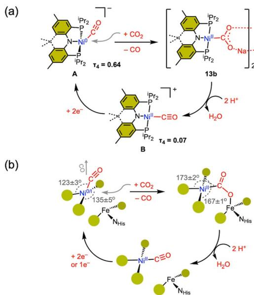
Fig. 5 (a) Synthetic cycle for CO<sub>2</sub> to CO in the (<sup>acri</sup>PNP)Ni system. (b) Proposed CODH mechanism based on the model study; bond angles are based on Table 1.
