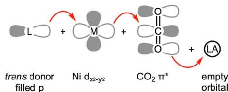
Fig. 4 Frontier orbitals involved in CO<sub>2</sub> activation.
