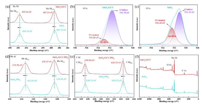
Fig. 2 XPS high-resolution spectra of  $SnO_2/GCC$  for (a) Sn 3d and (b) and (c) O 1s. XPS high-resolution spectra of  $SnO_2/Pbl_2$  and  $SnO_2/GCC/Pbl_2$  for (d) Pb 4f and (e) I 3d. (f) XPS full spectra of  $SnO_2/GCC$ .
