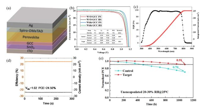
Fig. 6 (a) Schematic illustration of an implemented PSC. (b) J-V curves of the PSC device with and without GCC treatments. (c) The EQE spectrum and integrated current of the PSC device after GCC passivation. (d) Steady-state power output curves of PSCs. (e) The environmental stability curves of the control and GCC-modified unencapsulated devices at 20-30% RH @ 25 °C.
