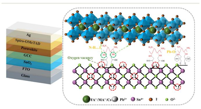
Fig. 1 A schematic diagram of the modification mechanism of GCC at the ETL/perovskite interface is proposed. The chemical structure of the GCC molecule is shown in the middle of the diagram.
