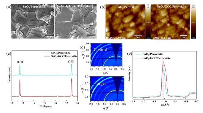
Fig. 4 (a) SEM and (b) AFM images of perovskite films deposited on SnO<sub>2</sub> and SnO<sub>2</sub>/GCC ETLs. (c) XRD patterns of perovskite films. (d) 2D-GIWAXS images, and (e) derived 1D integral analysis spectra of the perovskite films deposited on SnO<sub>2</sub> and SnO<sub>2</sub>/GCC ETLs.
