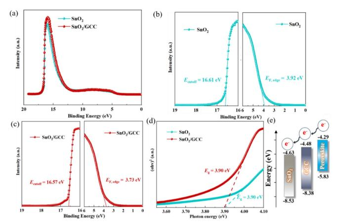
Fig. 3 (a) UPS full spectra of SnO<sub>2</sub>/GCC. UPS spectra of (b) SnO<sub>2</sub> film and (c) SnO<sub>2</sub>/GCC film. (d) Tauc-plot spectra of perovskite films deposited on SnO<sub>2</sub> and SnO<sub>2</sub>/GCC substrates. (e) The energy level diagram of SnO<sub>2</sub>, SnO<sub>2</sub>/GCC, and perovskite.
