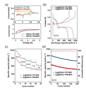
Fig. 5 Electrochemical performance of 2D PAV-S<sub>8</sub> composites as electrodes. (a) CV curves of various composites (60 wt% sulfur, top) and pristine 2D PAVs (down). (b) GCD curves of S<sub>8</sub>@2DPAV-TPB-BPZ and  $S_8@2DPAV-TPT-BPZ$  with 86 wt%  $S_8$ . (c) Rate performances. (d) Cycling performance. All the gravimetric discharge capacities are calculated based on sulfur.
