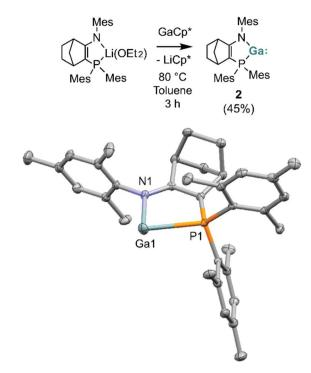
Fig. 4 Synthesis of gallylene 2. X-ray structure of 2 (H atoms omitted for clarity). Thermal ellipsoids at 50% probability. Selected bond distances (Å) and angles (°): Ga1–N1 1.962(2), Ga1–P1 2.7093(5), N1–Ga1–P1 78.92(5).
