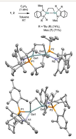
Fig. 8 Synthesis of compounds 6 and 7 (top). X-ray structures of compounds 6 and 7 (H atoms omitted for clarity). Thermal ellipsoids at 50%. 6: Ga-Ga 2.4799(7) Å, Ga-C 2.027(4)-2.043(4) Å; 7: Ga-Ga 2.5011(8) Å, Ga-C 2.023(5)-2.031(5) Å.
