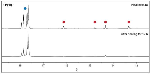
Fig. 9 Reversible ethene binding to 1 (top).  $^{31}P\{^1H\}$  NMR spectra showing thermally induced conversion of *syn* isomers **6D**–**F** to *anti* isomers **6A**–
