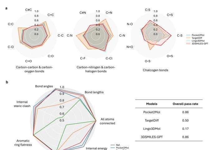
Fig. 2 Quality of generated conformations. (a) The Jensen–Shannon Divergence (JSD) of common chemical bond lengths between 3DSMILES-GPT and other models, compared to reference molecules. For ease of visual comparison, the values are presented as 1-JSD, where values closer to 1 indicate better performance. (b) The performance on each metrics and the overall pass rate of each model tested with PoseBusters.
